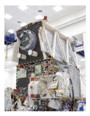
**Figure 15.** ATLID integrated on EarthCARE satellite platform. Reproduced with permission of Airbus ©.
