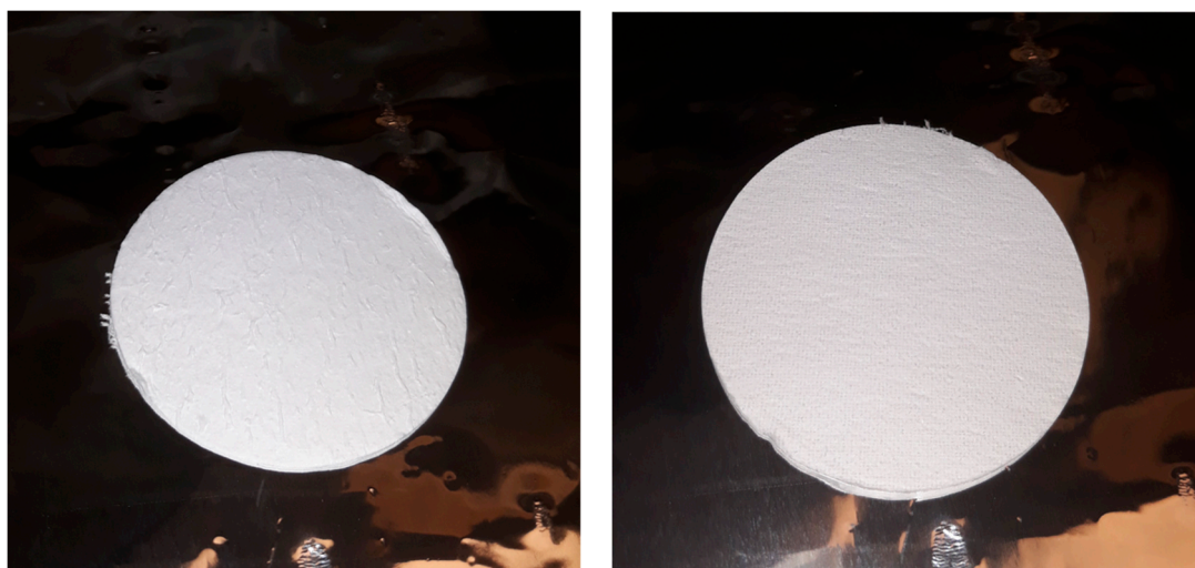
Figure 2. A filter right side up (left picture) and wrong side up (right picture).
