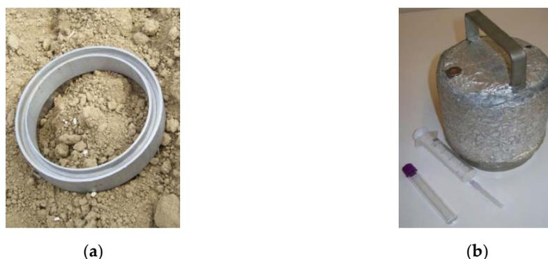
**Figure 1.** Metal ring permanently installed on the field (a) and closed-chamber, air syringe with needle, and vacuum test tube (b).
