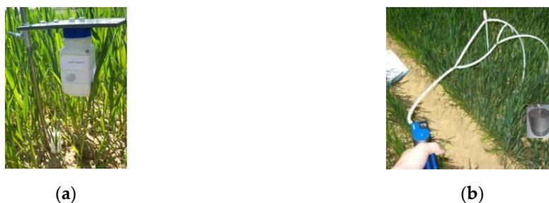
**Figure 2.** Passive-flux-collector from a square bottle with a modified acid trap for NH<sub>3</sub> (a) and Dräger-Tuber method (DTM) with Teflon tubes for hand pumping (b).
