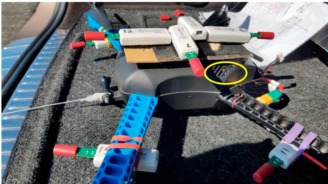
**Figure 8.** Photograph of the UAV showing the battery compartment vent on the left side of the UAV (yellow ellipse) towards the rear of the UAV, and the locations of several iMET-XQ sensors.
