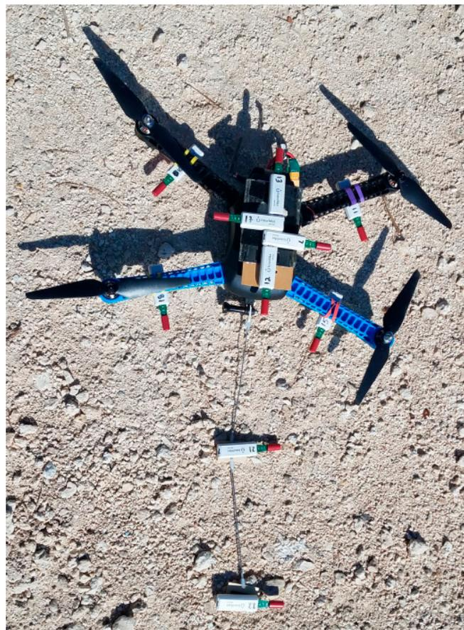
**Figure 1.** Photo of the Iris+ quad-copter with all 10 iMET-XQ sensors.
