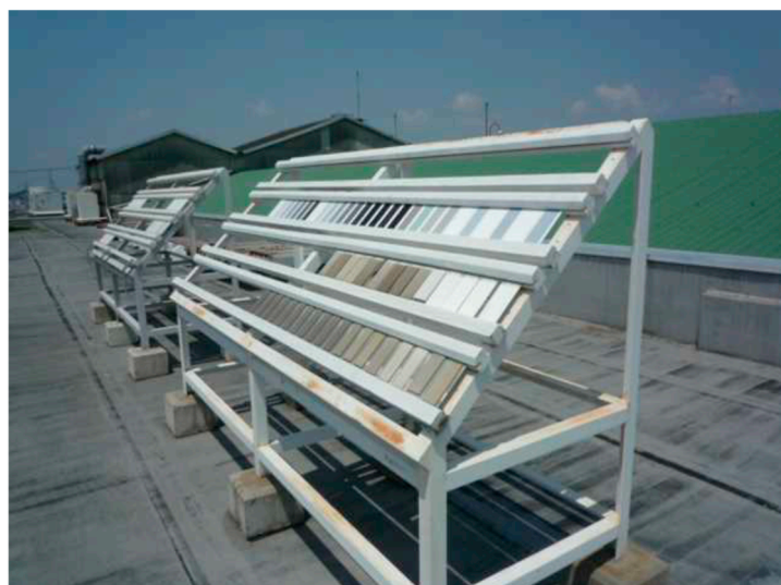
Figure 3. Outdoor exposure test at Osaka.
