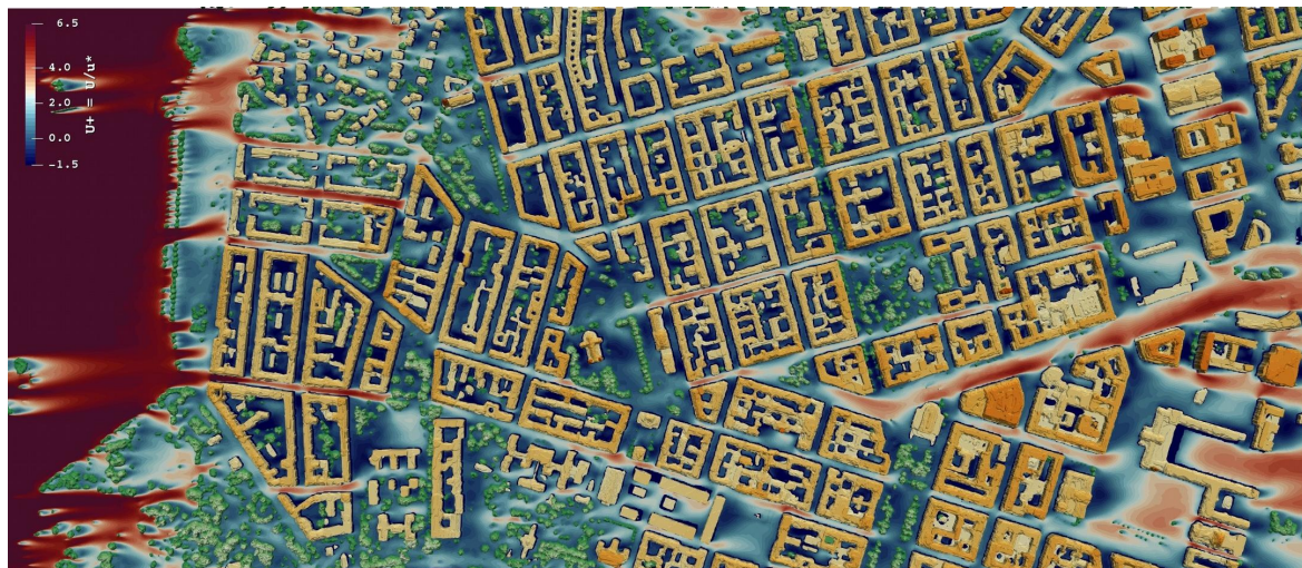
Figure 6. Horizontal distribution of \bar{u}_1^+ at z/H = 0.7 from case [R] across the urban area within the \Omega^{(2)} domain featuring \Delta = H/10 resolution.
