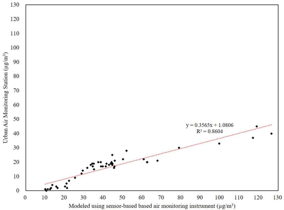
**Figure 6.** Correlation between outdoor PM<sub>2.5</sub> concentrations measured by the Urban Air Monitoring Station and modeled by sensor-based air monitoring instruments in Guro-gu.
