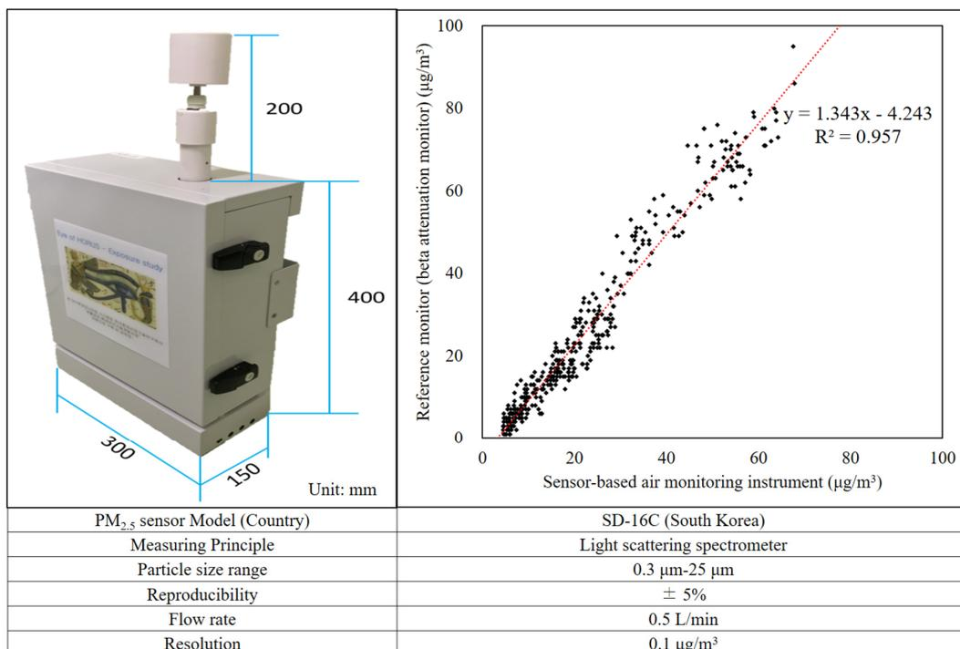
Figure 2. Specification of sensor-based air monitoring instrument.
