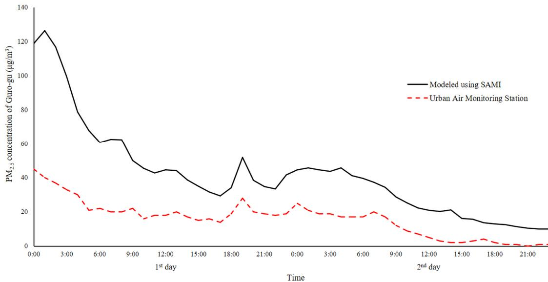
**Figure 4.** Comparison of outdoor fine particulate matter ( $\text{PM}_{2.5}$ ) concentrations modeled by a sensor-based air monitoring instrument (SAMI) and measured by an urban air monitoring station over time.
