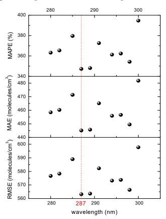
**Figure 6.** SO<sub>2</sub> single-wavelength error distribution. The red dot line indicates that the inversion using wavelength of 287 nm has the smallest error.
