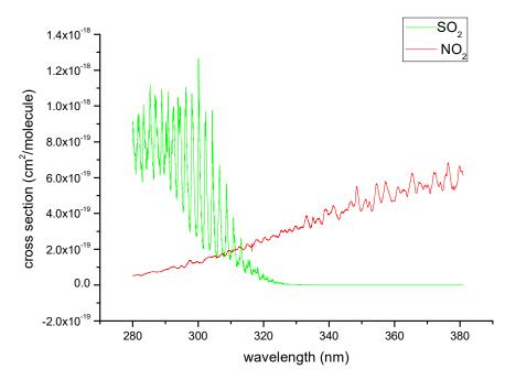
**Figure 1.** SO<sub>2</sub> absorption cross-section and NO<sub>2</sub> absorption cross-section (data source: The HITRAN 2016 molecular spectroscopic database [21]).
