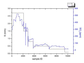
Figure 4. Changes in SO<sub>2</sub> concentration and sulfur content with time.
