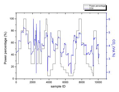
Figure 5. Changes in  $CO_2$  concentration and engine load with time.
