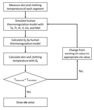
**Figure 2.** Flowchart of the evaluation of the clothing thermal insulation (clo level) using the human thermoregulation model.
