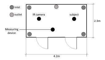
Figure 3. Floor plan of the climate chamber.
