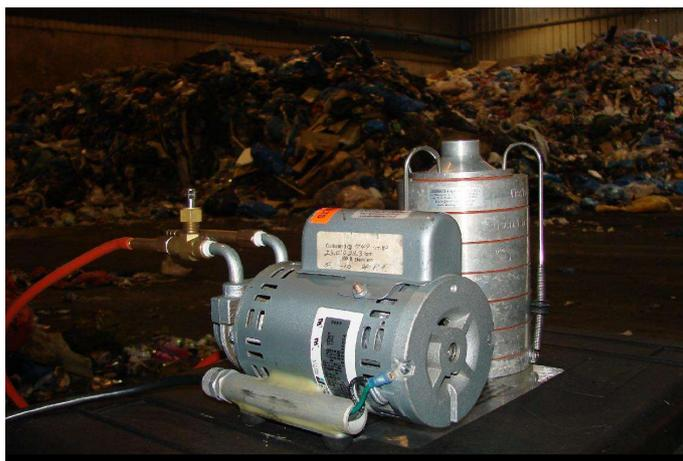
**Figure 2.** Six-stage Andersen impactor used during measurements in the waste sorting plant.
