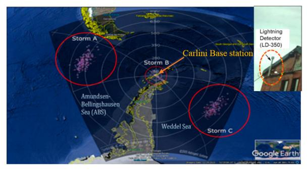
**Figure 2.** Locations and areas of lightning strokes detected by the lightening detector (LD) system installed at the Carlini Base, Antarctic Peninsula (Figure © 2019 Google Earth).
