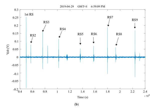
**Figure 3.** The RS captured by the (**a**) fast antenna (FA) system and (**b**) the expanded view of the fast field signal.
