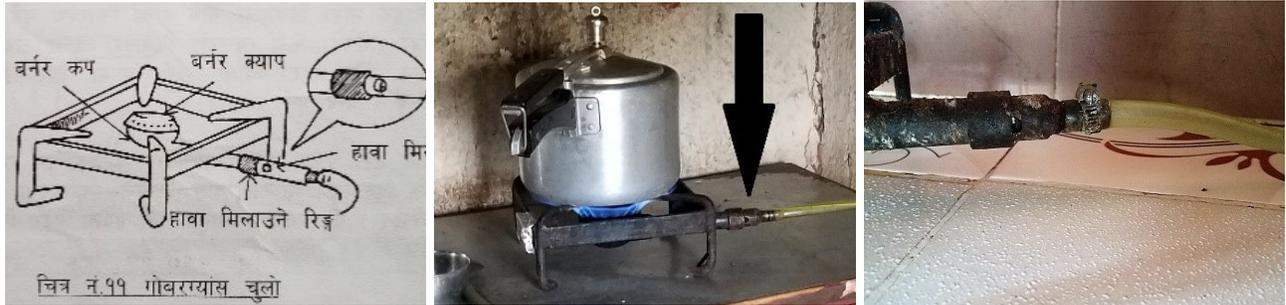
Figure S4: Biogas air inlet valve. Left: biogas system instruction manual describing the primary air valve control. Center: biogas stove with primary air valve half open. Right: close-up of primary air valve half open
