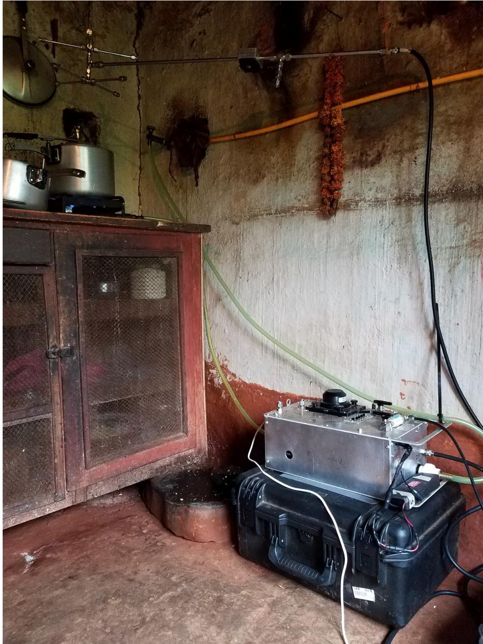
Figure S7: Emission and fuel gas measurements from a biogas stove.
