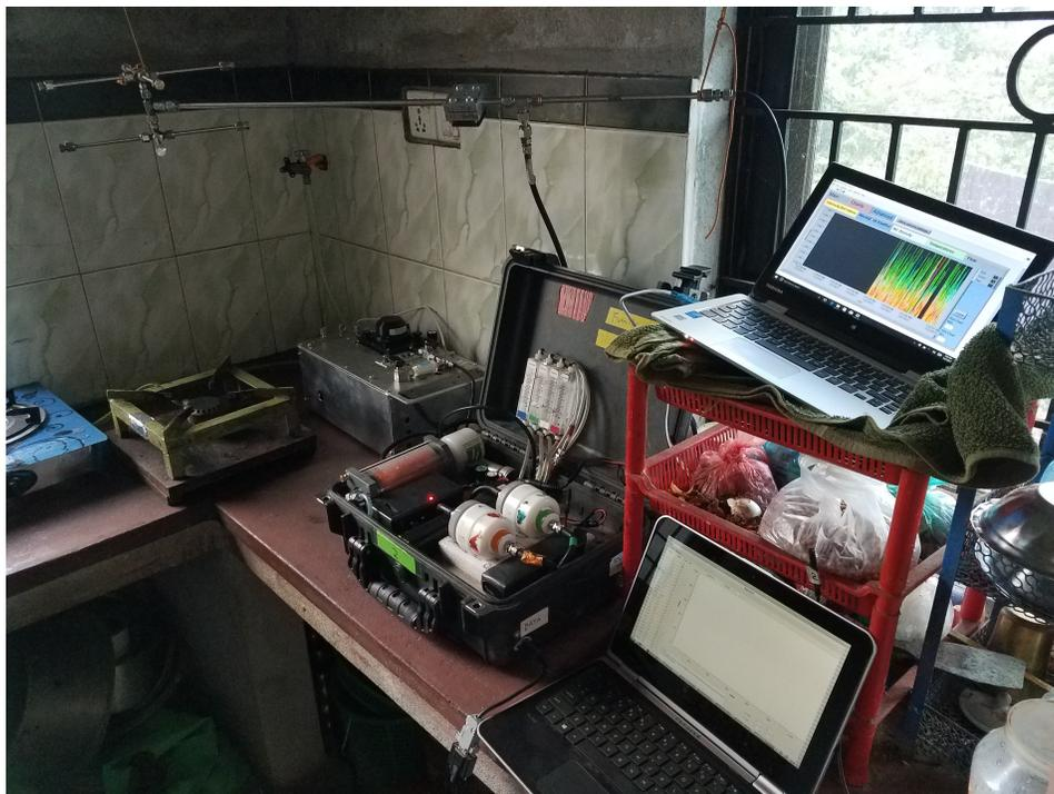
Figure S8: Emission and fuel gas measurements from a biogas stove.
