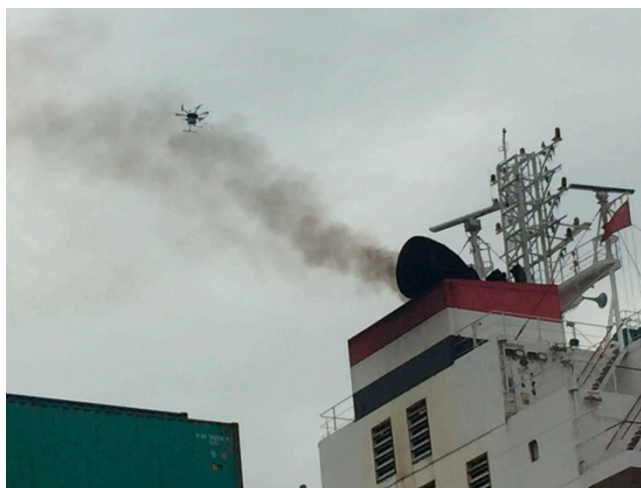
Figure 5. Photograph showing the flight of the rotary unmanned aerial vehicle during measurements.
