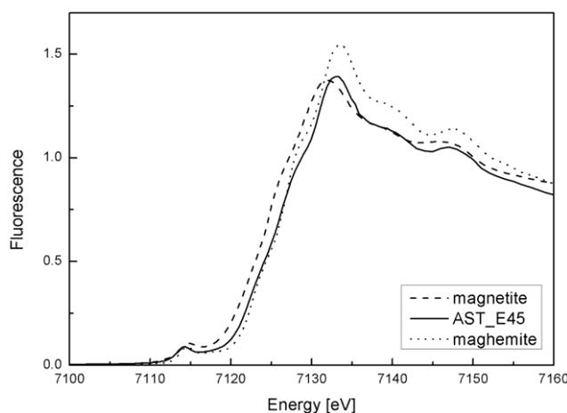
Figure S4 - Comparison between the AST\_E45 sample and magnetite and maghemite standards in the XANES region
