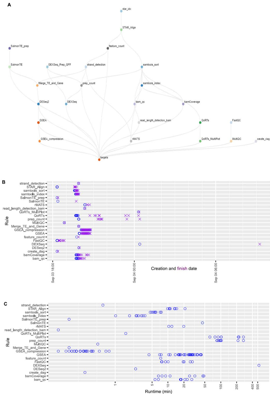
**Figure 6.** The structure of the OneStopRNAseq workflow and runtime statistics of each job. (A) A directional acyclic graph (DAG) showing the structure of the workflow. Jobs at lower levels depend on connected jobs at higher level and the workflow is executed from the top to the bottom following the specified job dependencies. (B) Creation and finish dates of each job. Blue circles indicate job creation dates and purple crosses show job finish dates. (C) Runtime of each job in minutes.
