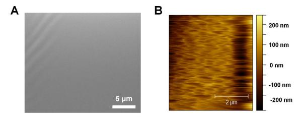
**Figure S1. The roughness characterization of fabricated polydimethylsiloxane (PDMS) structure. (A)** The enlarged SEM images of the curved tubule shows the smooth surface. **(B)** The curved surface roughness measurement by atomic force microscopy.
