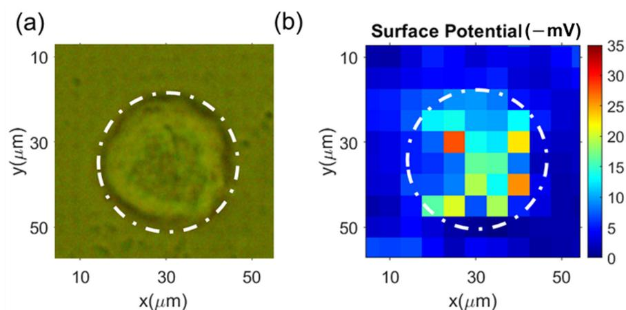
**Figure 6.** Typical measurement results of the surface charge mapping of HDFs: (a) optical images (top illumination) of the cells on the microelectrode array; (b) the corresponding surface charge mapping from the reflected images (measured from the back side of the microelectrode chip).
