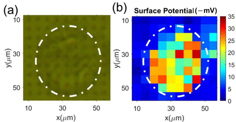
**Figure 7.** Typical measurement results of the surface charge mapping of hMSC: (a) optical images (top illumination) of the cells on the microelectrode array; (b) the corresponding surface charge mapping from the reflected images (measured from the back side of the microelectrode chip).
