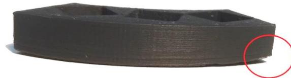
**Figure 3.** Warping in ABS printout circled in red.
