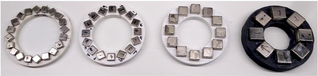
**Figure 6.** Halbach arrangements of 10, 12, 15, and 20 mm cubic magnets.
