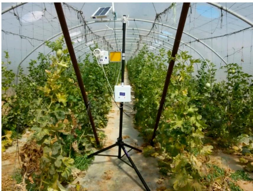
**Figure 6.** Image of a RETIC-Real Time Insect Counting Trap, wireless, monitoring system in the gate of a melon growing greenhouse in Ein Yahav, Arava Valley, during the spring of 2015.
