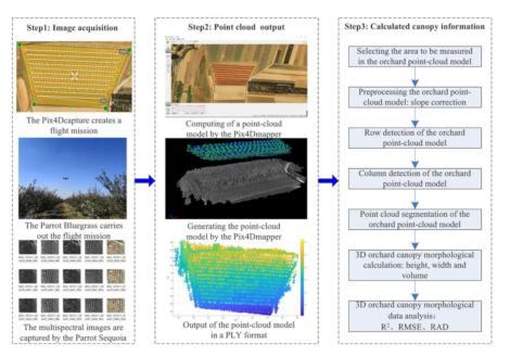
**Figure 1.** Operating principle of the UAV canopy photogrammetry system for modern standard orchards.
