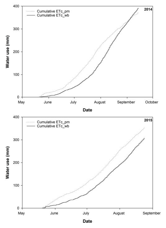
**Figure 2.** Cumulative crop evapotranspiration (mm) from FAO Penman–Monteith (ETc-pm) and water balance equations (ETc-wb) in 2014 and 2015.
