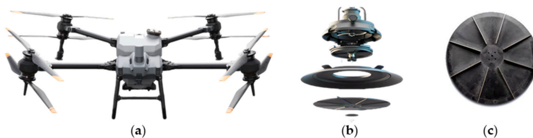
Figure 1. DJI T40 UAV Centrifugal Spreading System. (a) DJI T40 UAV Complete Machine Schematic; (b) Spreading System Component Decomposition; (c) Centrifugal Disc Structure.
