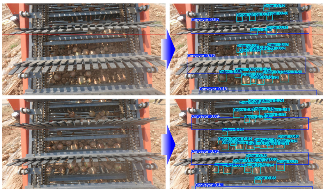
Figure 12. Representative object detection results overlaid on camera images of the collection unit during field operation.
