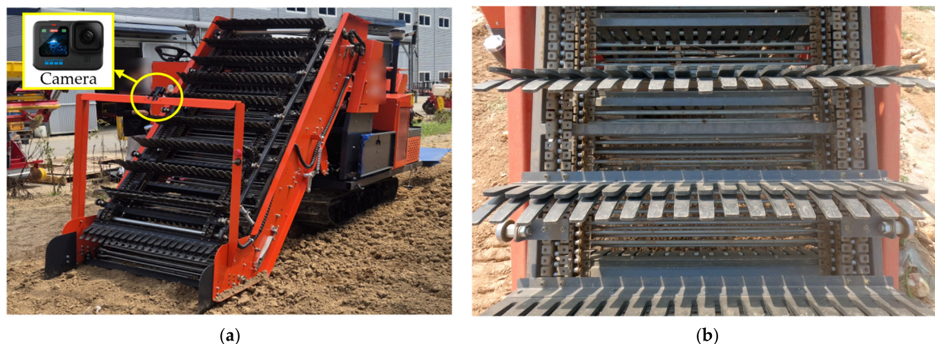
Figure 2. Photographs of the self-propelled onion collector: (a) Side view showing the camera installation position; (b) View of the collection unit captured by the installed camera.
