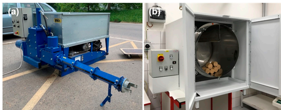
Figure 2. Briquetting press (a) and rotation drum (b).
