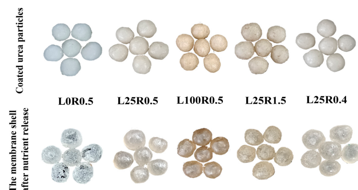
Figure 1. Picture of coated urea particles and picture of membrane shells after nutrient release.
