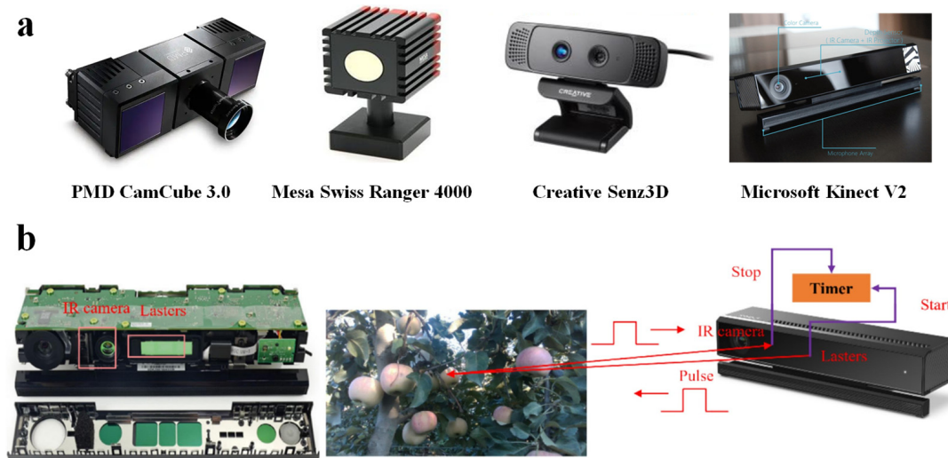
Figure 8. Time of Flight cameras: (a) examples and (b) principle [75].
