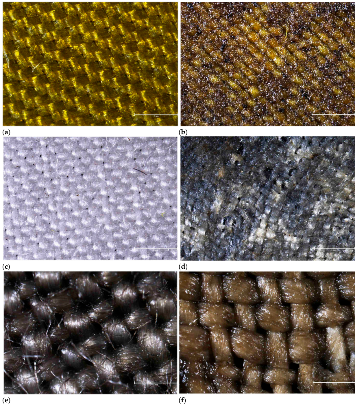
Figure 3. Microscopic images (30 \times ) of viscose, cotton, and linen textile samples under controlled composting conditions. (a) input material, viscose; (b) viscose residue after three months of controlled composting; (c) input material, cotton; (d) cotton residue after three months of controlled composting; (e) input material, linen; (f) linen residue after three months controlled composting. The scale bar of 1 mm is at the bottom right of each picture.
