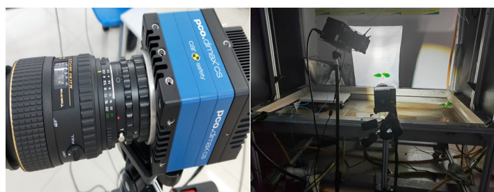
Figure 1. The droplet dynamic impact test system.
