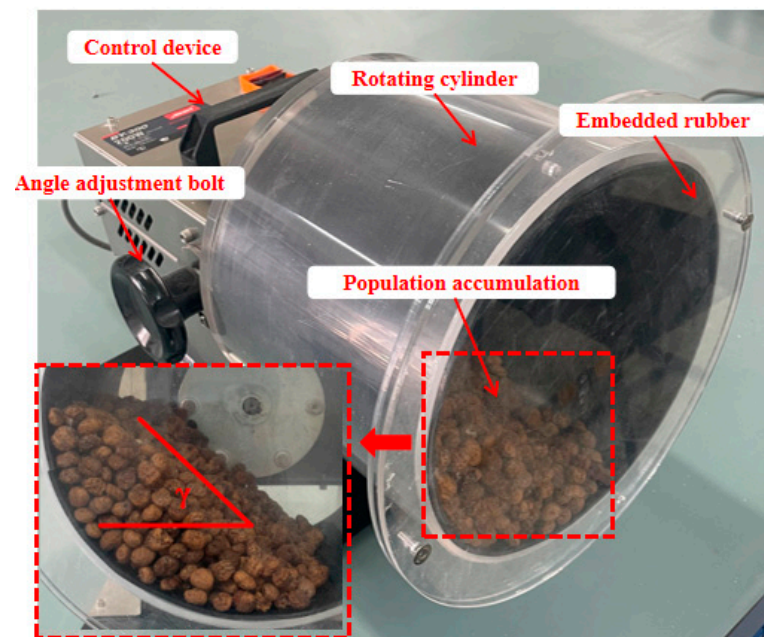
Figure 7. Physical Dynamic Stacking Angle Test.
