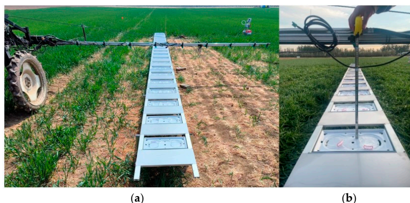
Figure 3. Test bench layout and boom height measurement: (a) Test bench layout; (b) measurement of boom height.
