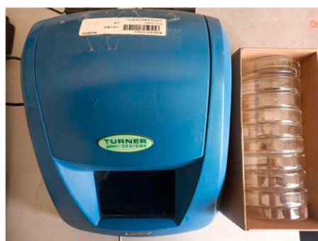
Figure 4. Trilogy 720-000 fluorometer and Petri dishes for testing.
