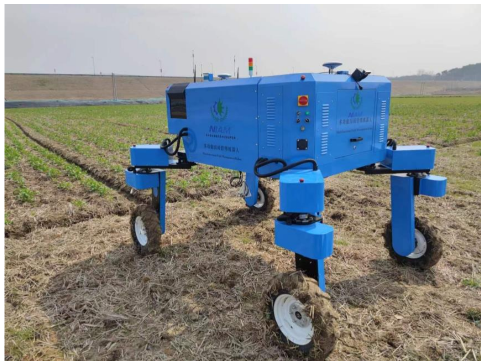
Figure 2. Agricultural robotics oilseed rape data collection platform.
