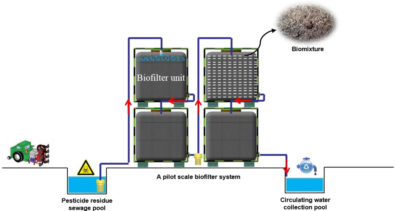
Figure 2. Operating diagram of the biofilter system.
