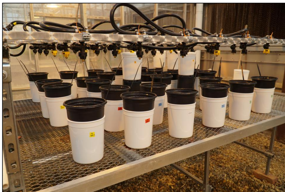
Figure 2. Photograph of Experiment 2 substrate containers, irrigation system, and leachate buckets. Photograph was taken prior to sheathing the white leachate buckets with black plastic.
