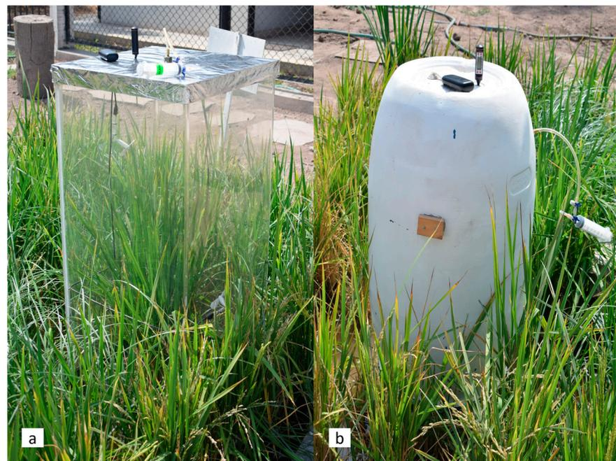
**Figure 6.** Closed static chambers in the field: transparent (a) and opaque (b).
