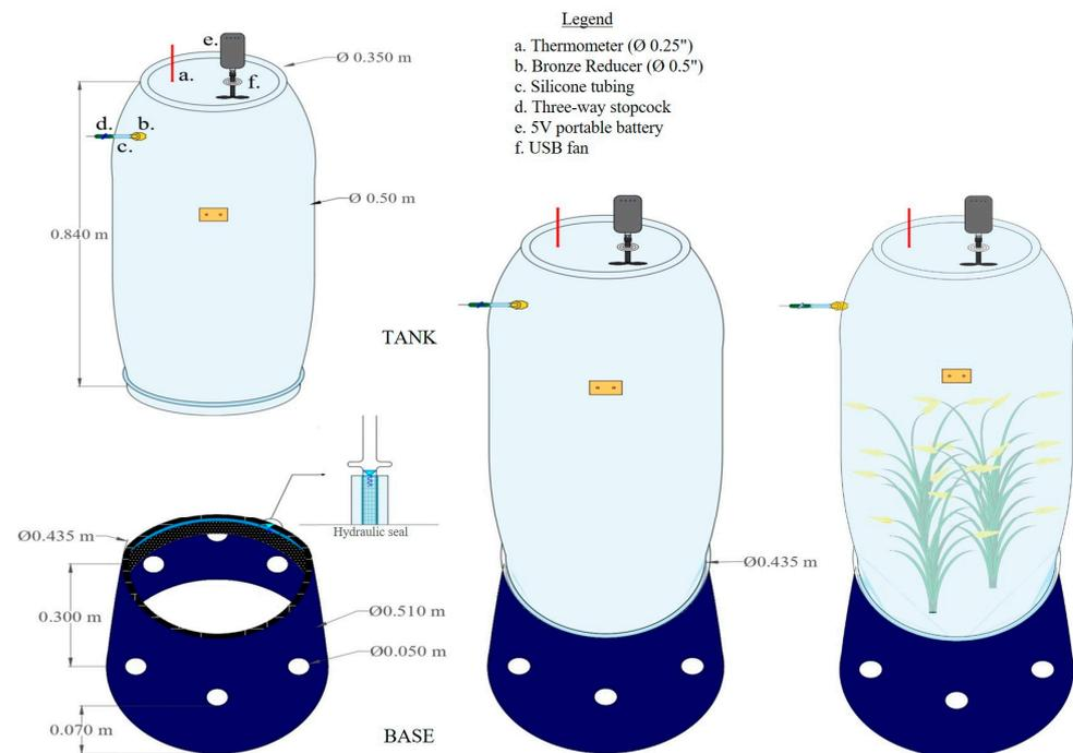
**Figure 4.** Diagram of the opaque closed static chamber.
