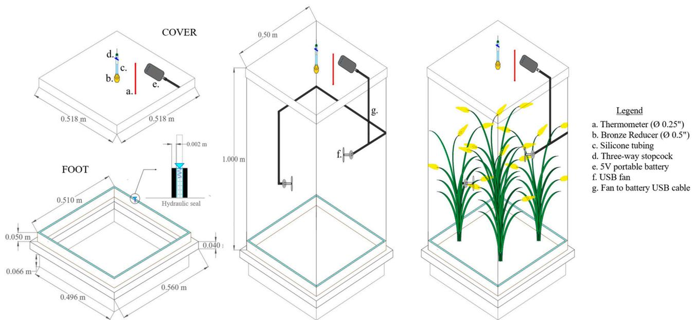
**Figure 5.** Diagram of the transparent closed static chamber.
