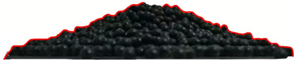
Figure 5. Cone image from laboratory repose angle test.
