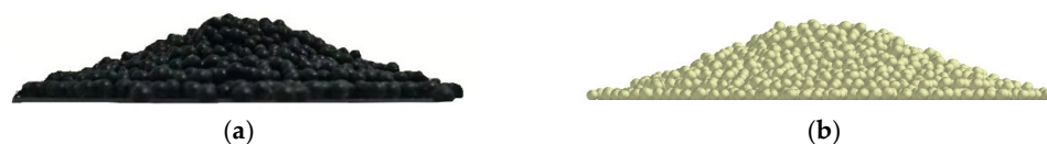
Figure 16. Verification of optimized DEM parameters: (a) repose angle measured in the laboratory. (b) Repose angle from the DEM simulation.
