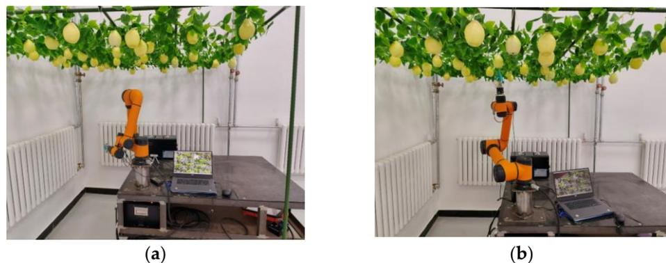
**Figure 21.** Picking diagram. (a) Initial pose; (b) target pose.
