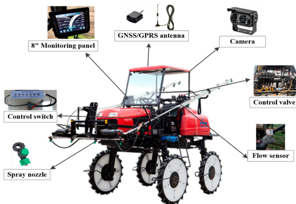
Figure 1. Autonomous intelligent crop protection machinery with precision spraying control system.
