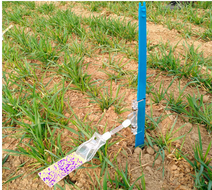
Figure 3. A device used for fixing the droplet measuring cards in the field. (The photograph was captured shortly after the spraying process).
