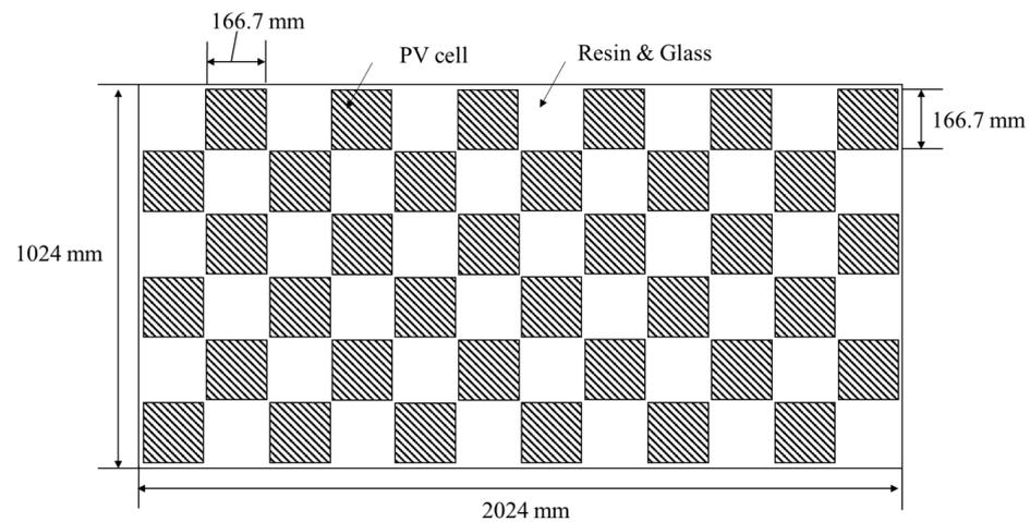
**Figure 11.** Devised semi-transparent building integrated photovoltaic.
