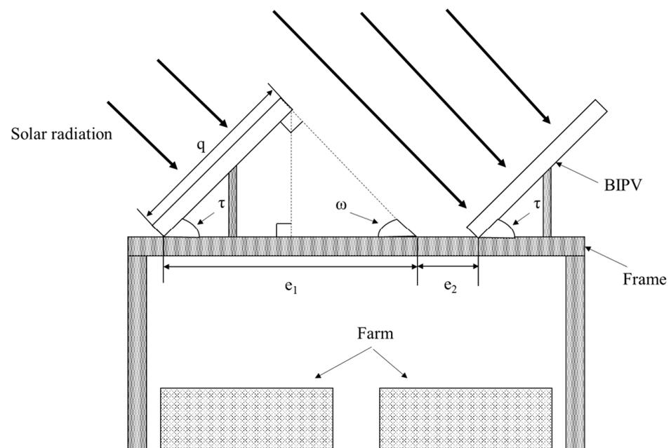
**Figure 6.** Design of the subject agrivoltaic system.
