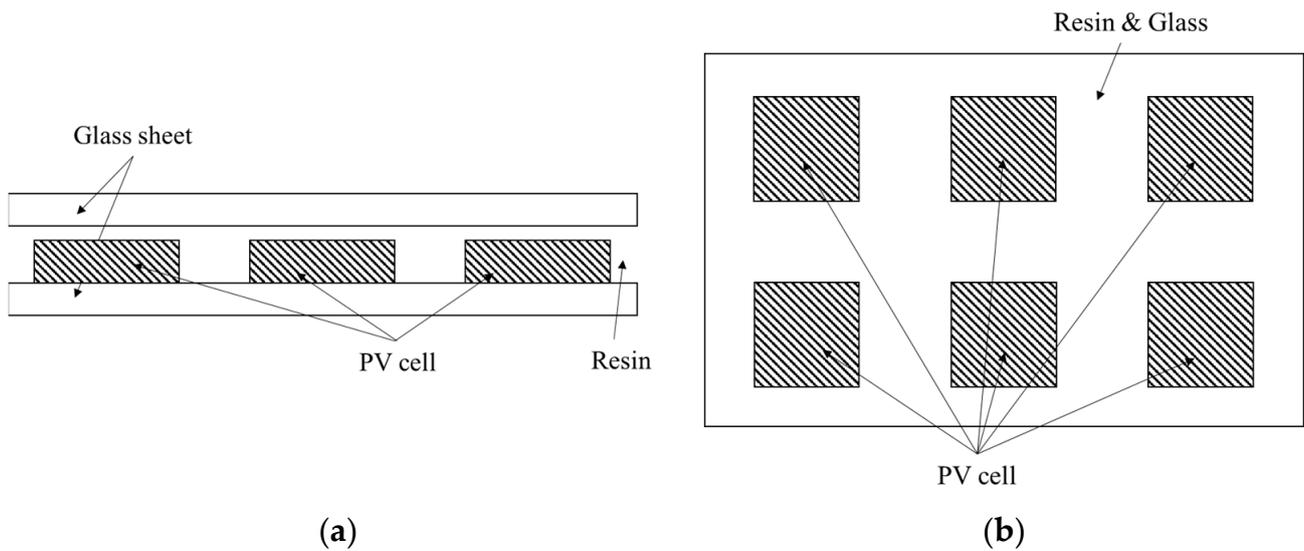
**Figure 3.** Structure of a semi-transparent building integrated photovoltaic (BIPV): (a) side view; (b) front view.
