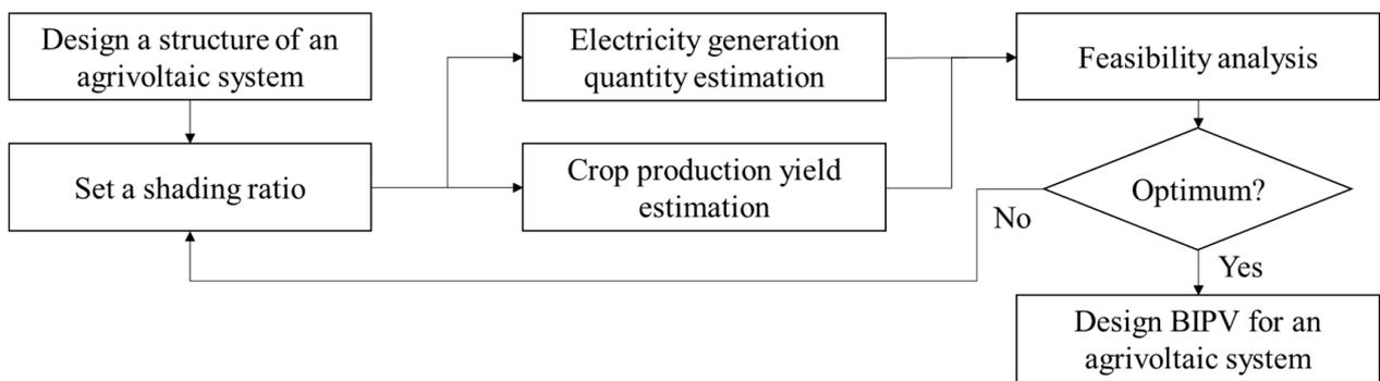
**Figure 4.** Proposed framework for agrivoltaic system design with building integrated photovoltaics.
