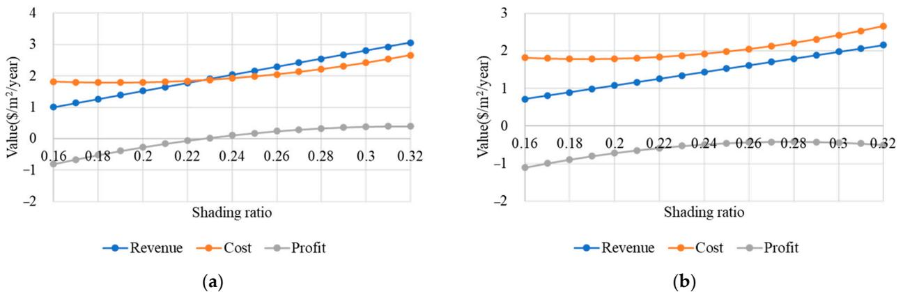
Figure 8. Revenue, cost, and profit of electricity generation: (a) REC and SMP case; (b) SMP case.
