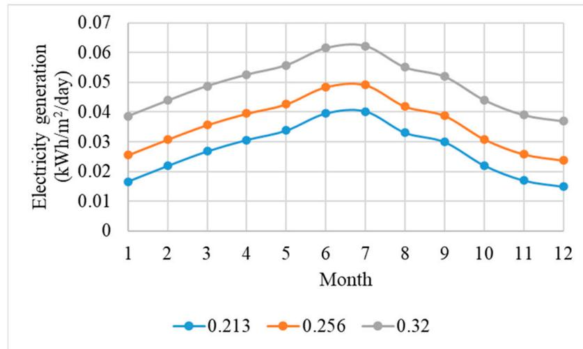
Figure 7. Electricity generation quantities under different shading ratios.
