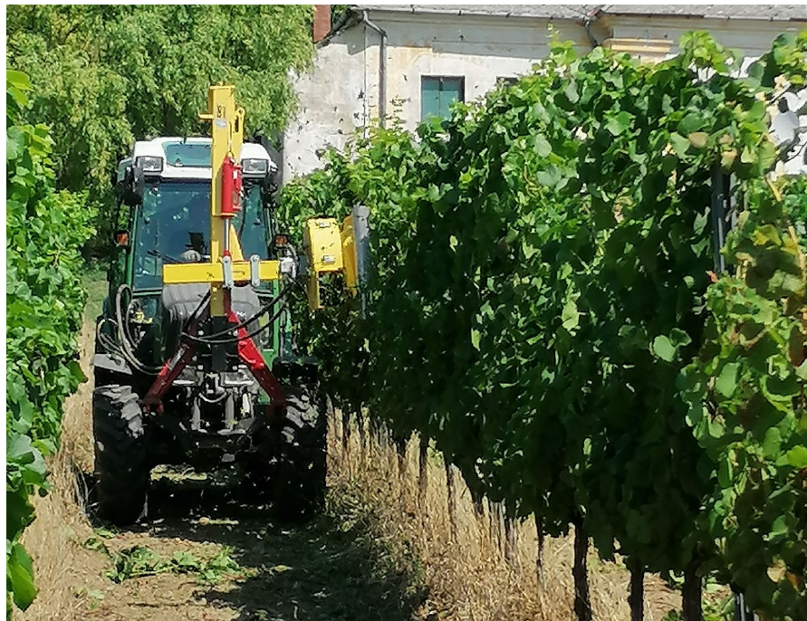
Figure 4. Mechanical leaf removal by tractor-mounted special leaf stripper machine.
