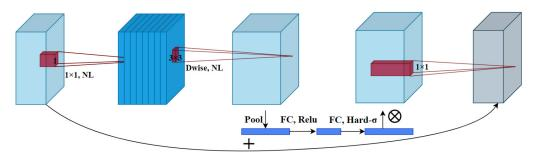
Figure 8. The MobileNetV3 base module.
