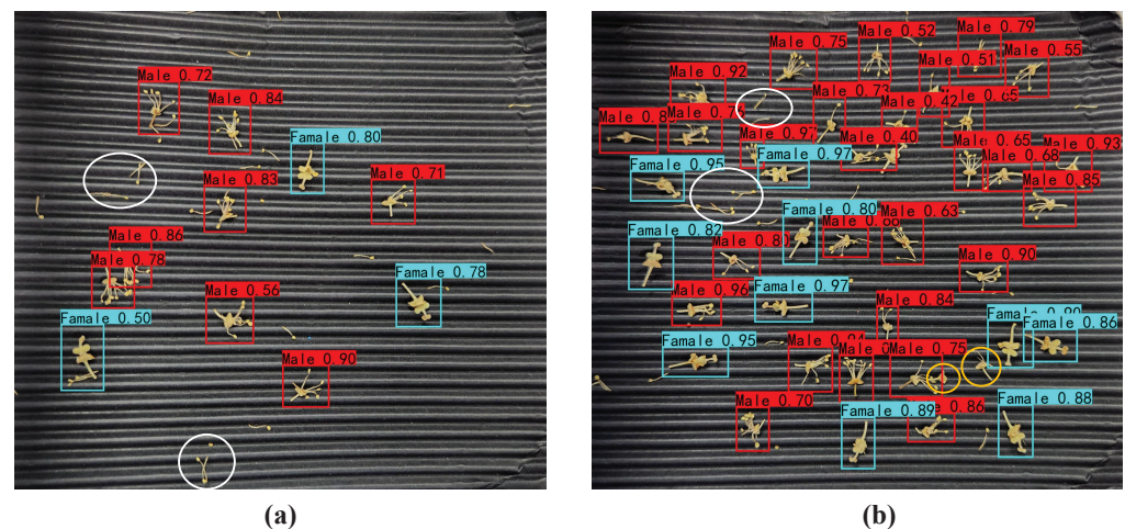
Figure 10. Test results of the model for the detection of male and female litchi flowers after distillation. (a) Sparse object. (b) Intensive object.
