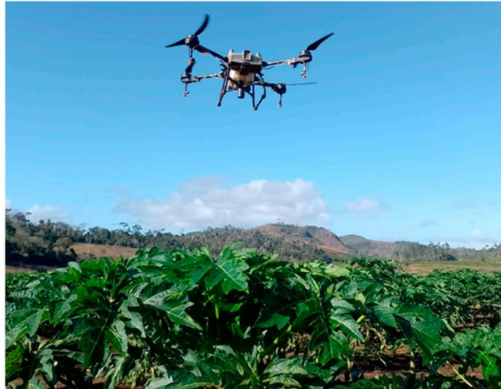
**Figure 2.** Multi-rotor unmanned aerial vehicle used in the spraying experiment.
