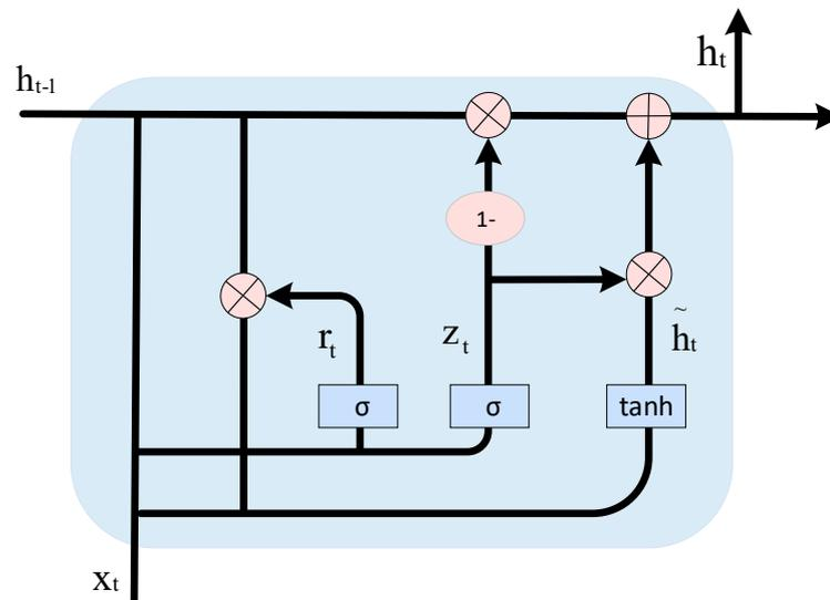
**Figure 3.** Internal unit structural diagram of GRU model.
