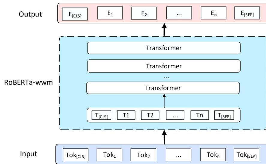
Figure 2. Structural diagram of RoBERTa-wwm model.
