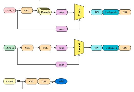
Figure 7. CSP module schematic.
