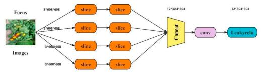
Figure 6. Focus module schematic diagram.
