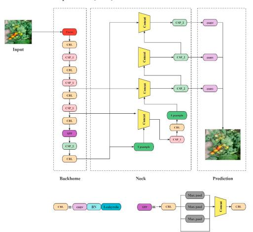
Figure 4. YOLOv5 network model structure diagram.
