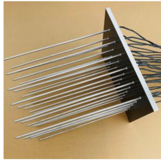
Figure 1. PT100 soil internal temperature acquisition device.
