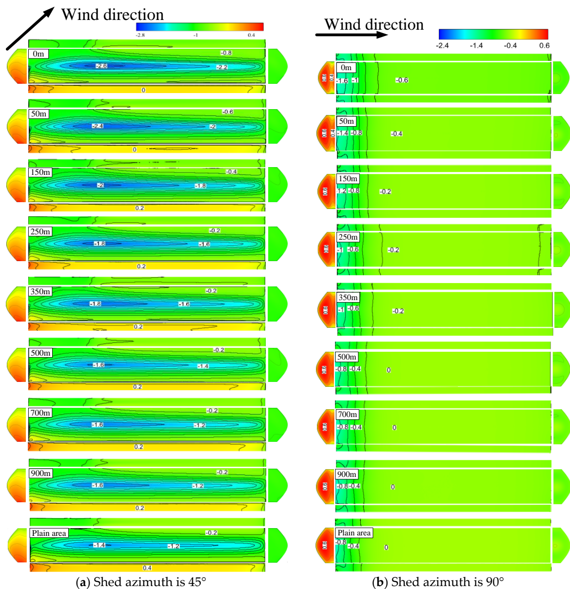
Figure 13. Wind pressure distribution of shed with d = 0, 50, 150, 250, 350, 500, 700 , and 900 m and in a plain area.
