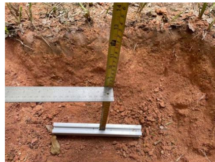
Figure 9. Field electromagnetic wave velocity measurement.
