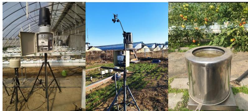
**Figure 2.** Meteorological stations inside the greenhouse and meteorological stations outside the greenhouse, as well as the evaporation pan.
