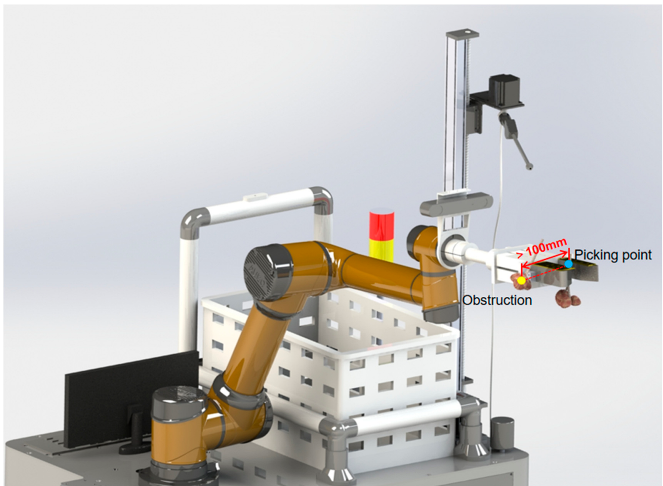
Figure 10. Diagram of the end-effector entering the space between the picking point and the obstruction.
