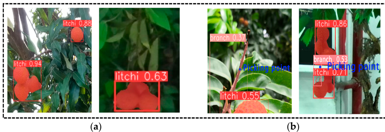
Figure 14. Two cases of failed recognition: (a) Unable to identify litchi branch; (b) picking point localization error.
