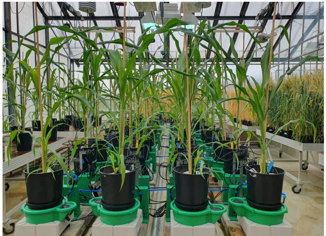
**Figure 3.** Plantarray, a high-throughput functional phenotyping (HTP) platform, was used in this study. Each pot is positioned on a sensitive load cell connected to the control unit.
